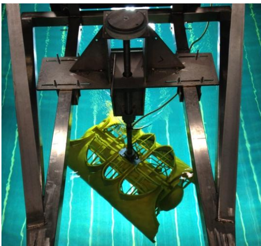
Figure 2 Captured testing of the model MWA setup (orientated at 45°)
